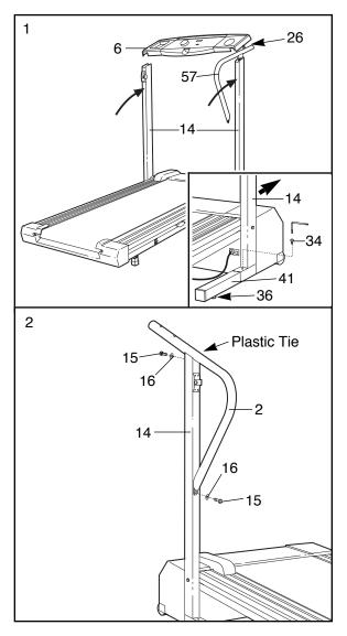
3. With the help of a second person, hold the Console Base (6) and the Right Handrail (57) near the right Upright (14) as shown. Insert all excess Wire Harness (26) into the Handrail and down into the right Upright. Bend the Wire Harness as shown, if necessary.
